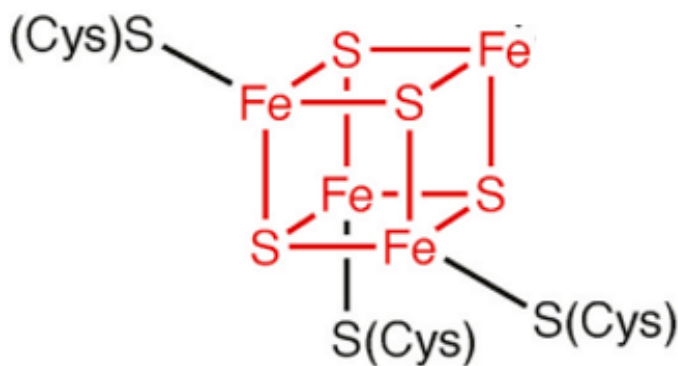
Figure 5: Iron-sulphur complex from aconitase, a [4Fe-4S] cluster.
